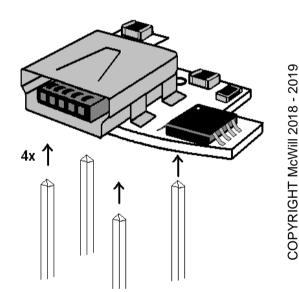
After soldering the pins to the USB charger PCB, you can put the USB charger PCB into the existing holes of the GBC power jack and solder them.
