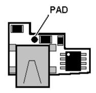
Finally solder 1 wire from the **PAD** of the USB charger PCB to the **battery clip** inside the **lower case**.
