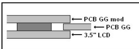
First solder 1 wire to **VCC** of the GG mod and 1 wire to **GND** of the GG mod and leave the other ends. Now slide the GG mod onto the Game Gear PCB and solder the 2 wires **VCC** and **GND** of the GG mod to the Game Gear PCB. **DON'T MIX THEM UP!!!** Solder 1 wire from **T10** to **T11** on the Game Gear Board.
